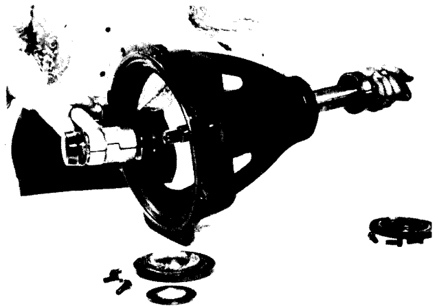
Fig. 16. Driving pump shaft from bearing bracket. (K-Frame shown)
