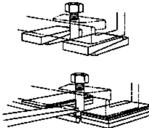
Figure 5. Unit Leveling
