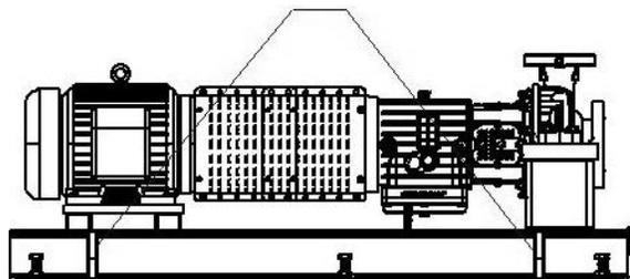
Fig. 2 Transport of the complete unit
