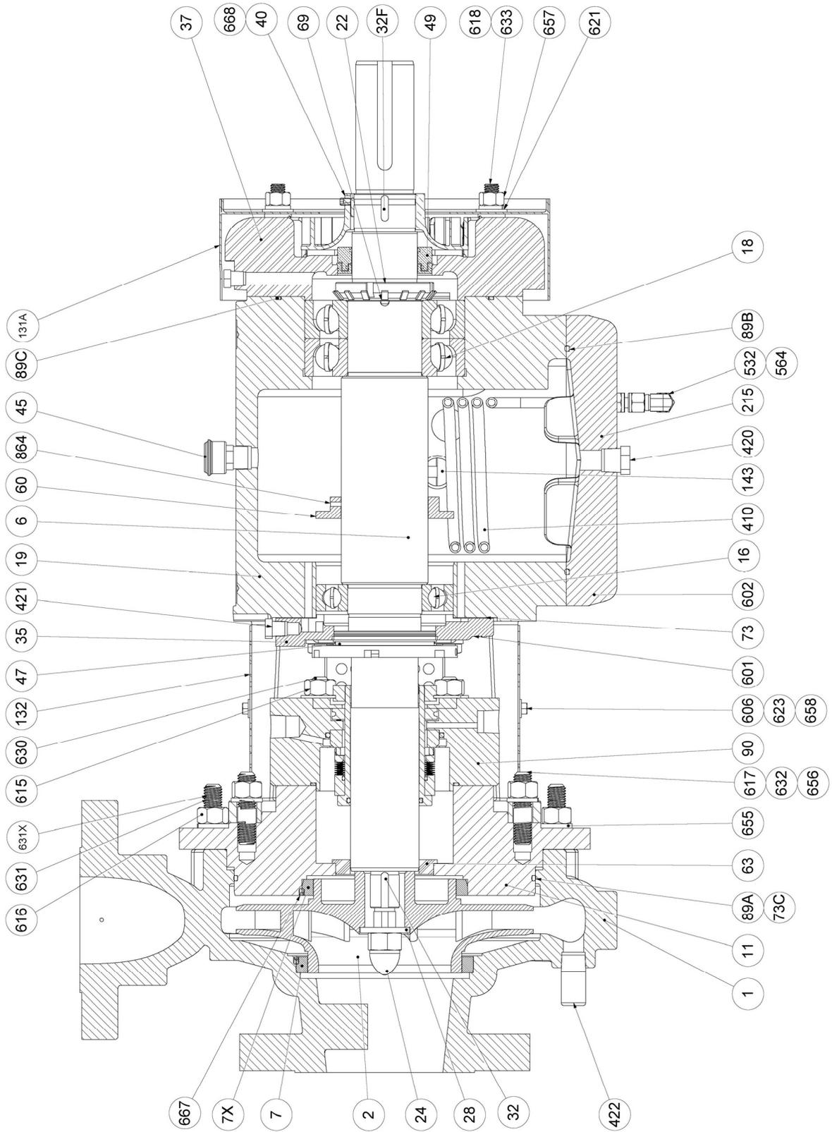
Figure 8 Sectional Assembly – Bare Pump
