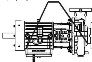
Fig. 1 Transport of the pump
