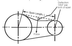
Figure 10. Belt Tensioning
