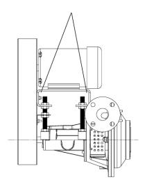
Figure 6. Transport of the complete unit
