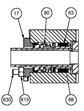
Figure 9. Mechanical Seal
