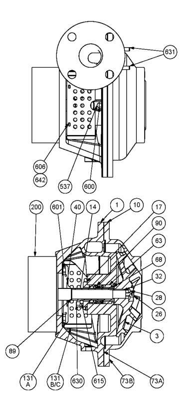
Figure 15. Sectional Assembly – Close-Coupled Pump (Shown with Mechanical Seal)
