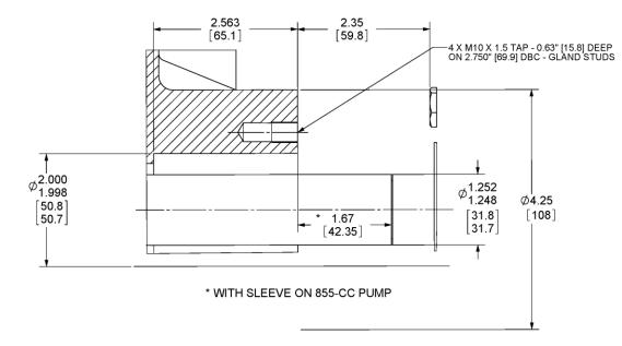
Figure 3. Stuffing Box Dimensions
