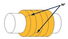
Figure 8. Packing Alignment
