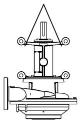
Figure 4. Transport of the bare pump
