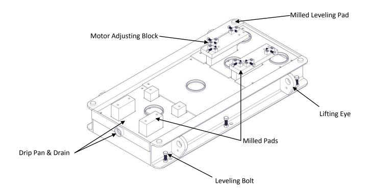
Figure 6. Unit Leveling
