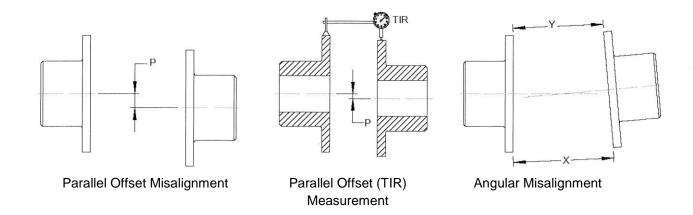
Figure 7. Coupling Alignment
