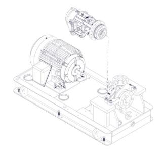
Figure 12. Remove back Pull-Out
