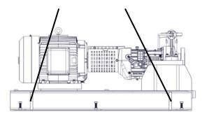
Figure 3. Sling Position for Moving Pumping unit
