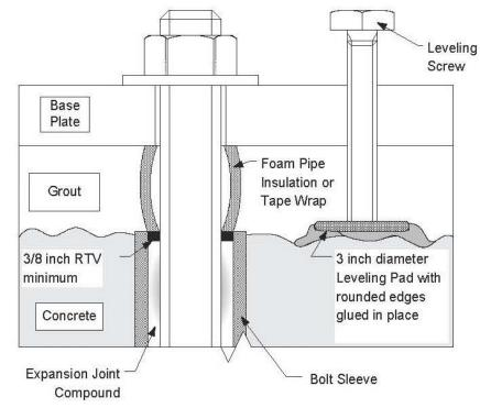
Figure 5. Grouting and Foundation Bolting
