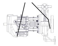
Figure 2. Sling Position for Moving Pump
